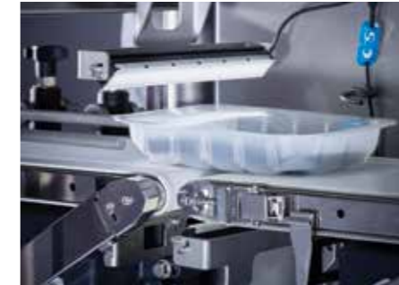
To fully monitor pack labels, a vision system can be mounted on the QC220 platform.
