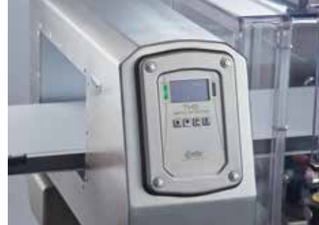
Metal detection: multi-frequency and multi-spectrum units can be integrated.
