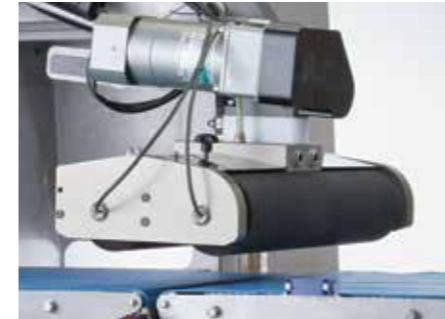
An underside conveyor is provided with the AirScan platform for sensing around the complete pack.
