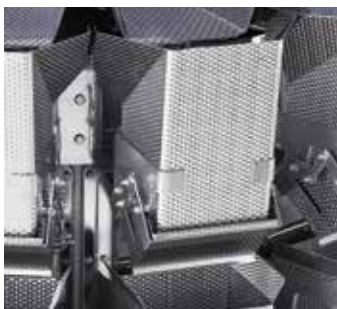
Faster opening and closing of hoppers
