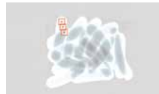
Final image processing The background product effect is further reduced enabling foreign bodies to be identified
