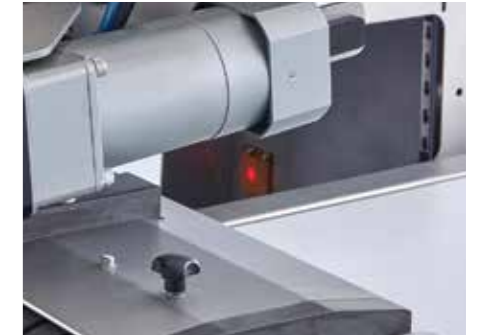
Bin full and reject confirmation sensors
