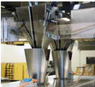
Two single twin timing hoppers deliver up to 400wpm
