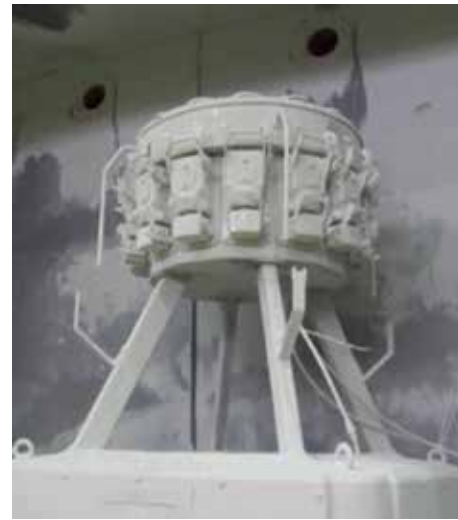
Dust test for IP6X
