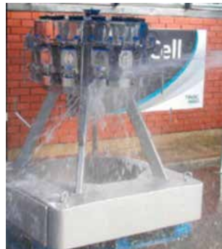
Under-going powerful water jet test for IPX6
