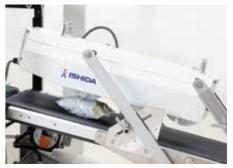
A variety of intake conveyors can be supplied to take packs from the bagmaker into the TSC seal tester
