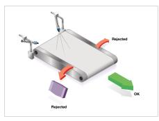
Air reject: best for high speed, relatively low-weight packs.
