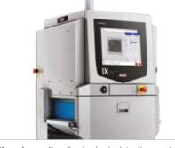
X-ray inspection: foreign body detection can be extended beyond metals by incorporating this increasingly in-demand technology.
