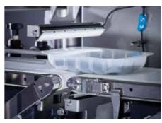
An underside conveyor can be provided with the AirScan platform for sensing around the complete pack
