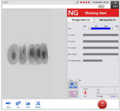
Example: Low custard filling detected in a finished pack of donuts
