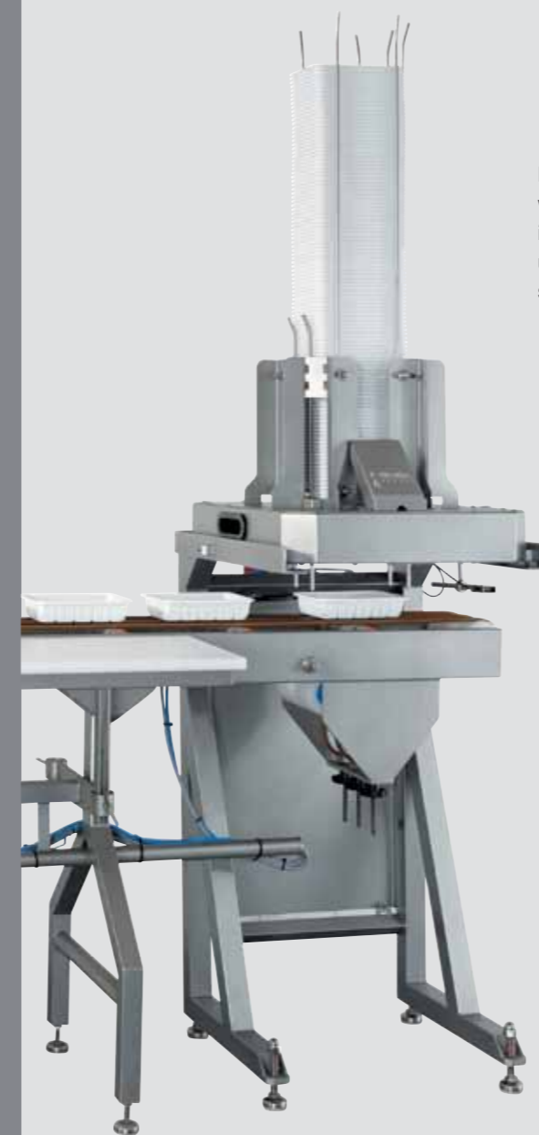
Fast, reliable denesting at 120+ trays per minute
