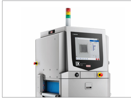
X-ray inspection: foreign body detection can be extended beyond metals by incorporating this increasingly in-demand technology.
