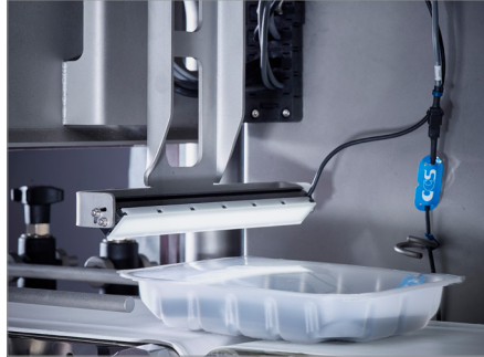
To fully monitor pack labels, a vision system can be mounted on the QC220 platform.
