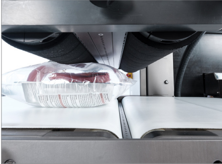
An underside conveyor is provided with the AirScan platform for sensing around the complete pack.
