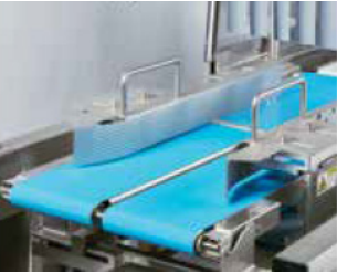
Spacing conveyor with motorised infeed guides
