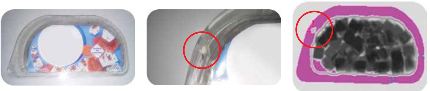
Fig.6: Trapped product detected in a seal of the tray with sliced feta cheese.
