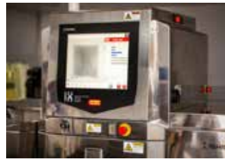
The X-ray system inspects pack of grated cheese.
