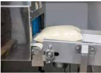
Pack of grated cheese enters X-ray inspection chamber.
